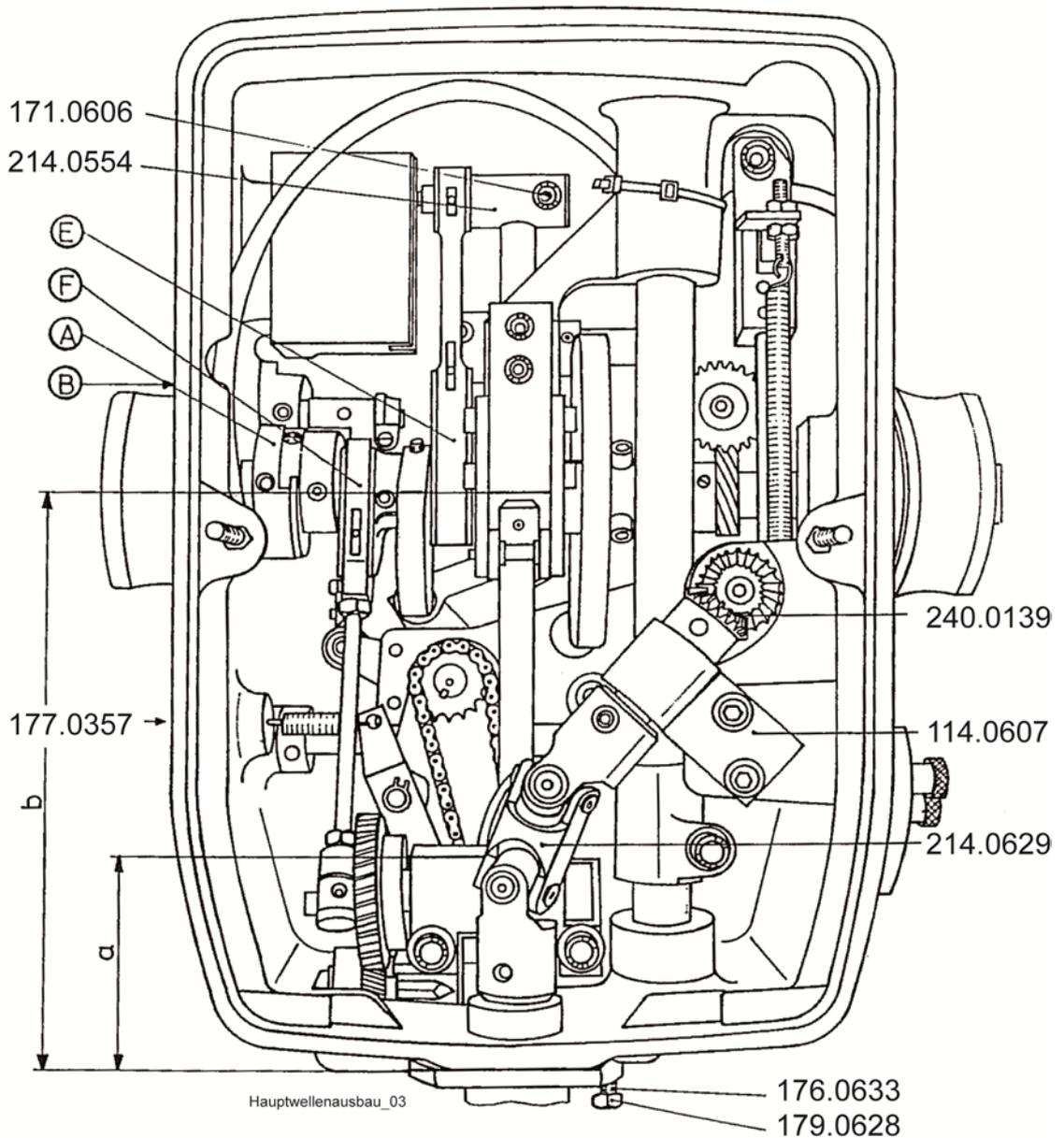
(Only) then loosen the screws of the parts on the shaft, remove the right hand wheel and push the shaft towards the left side by means of a pulling-off device without displacing the ball bearings.
