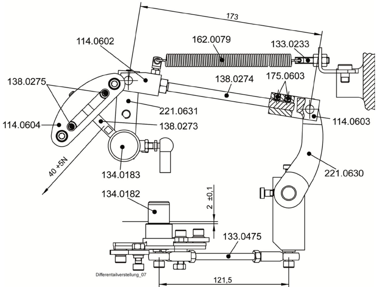
After mounting gear shifting gate 114.0604 with all belonging parts, trip dog 138.0275 may be adjusted provisionally. It should sit close to bolt 138.0273 when lever 221.0630 is in zero position. (Fig. 27)
