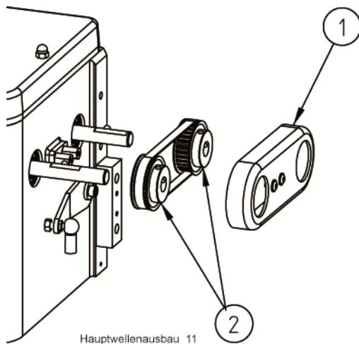
The left handwheel with the stitch variable eccentric bolt does not need to be removed. **Make sure** that the threaded pins (2) located on both sides of the variable eccentric (A) (1) are removed. (Fig. 4 and Fig. 5)
