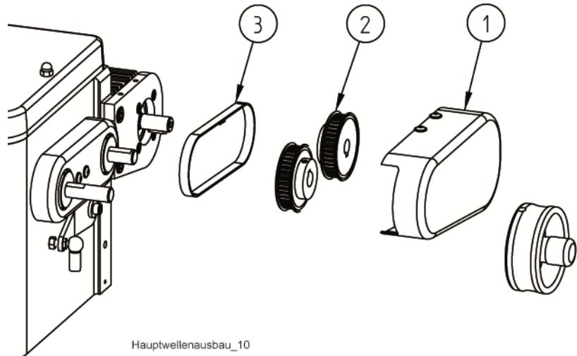
Afterwards the belt guard (1). Now make a note of how the two toothed belt pulleys (2) are mounted on the front and rear shaft. Now the toothed belt pulleys (2) can be taken off with the toothed belt. (Fig. 3)
