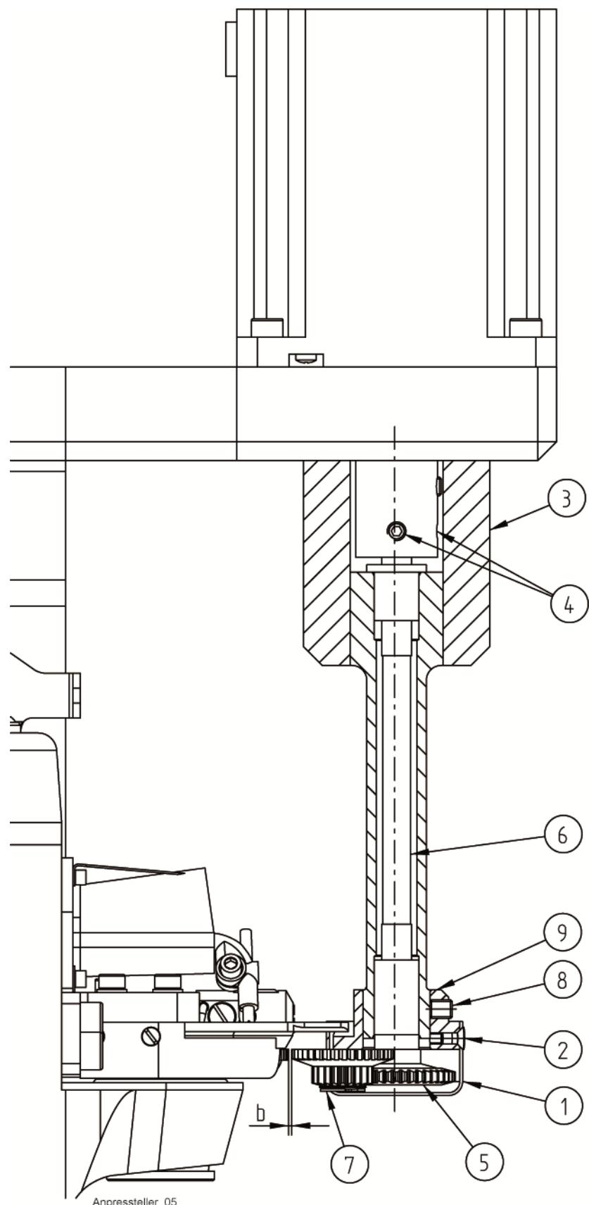
**4.8****Tread lifting in the needle bar head**
