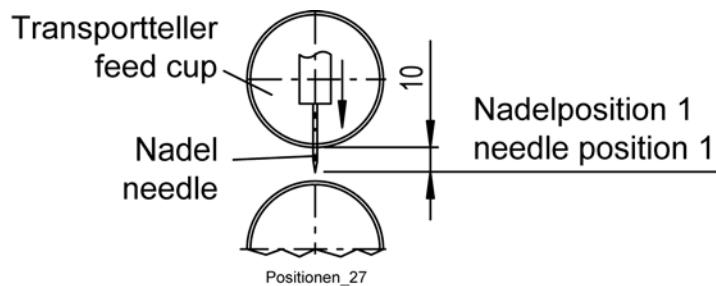
Needle position (when stop outside the stitch with pedal position "-2" (Fig. 18)):
