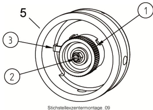
Screw the control knob (1) onto the shaft or the adjustment bolt (2) until the control knob contacts the handwheel. Hold the control knob tight and screw out the adjustment bolt until the pointer (3) on the control knob of the handwheel (marking 5), (large stitch), contacts and can be slightly seen between handwheel and stand. (Fig. 7)
