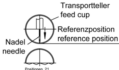
Refer to the enclosed sewing drive instructions for the programming of the positions on the motor.
