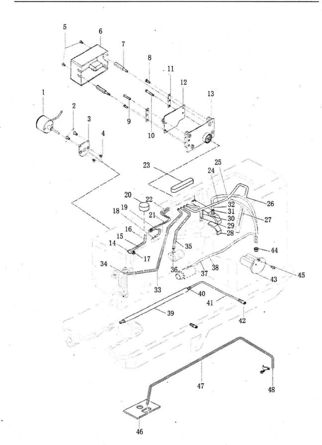
L. Tension release, electrocircuit board, oil circuit parts
