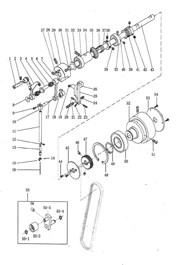
C. Arm shaft and needle bar thread take up parts
