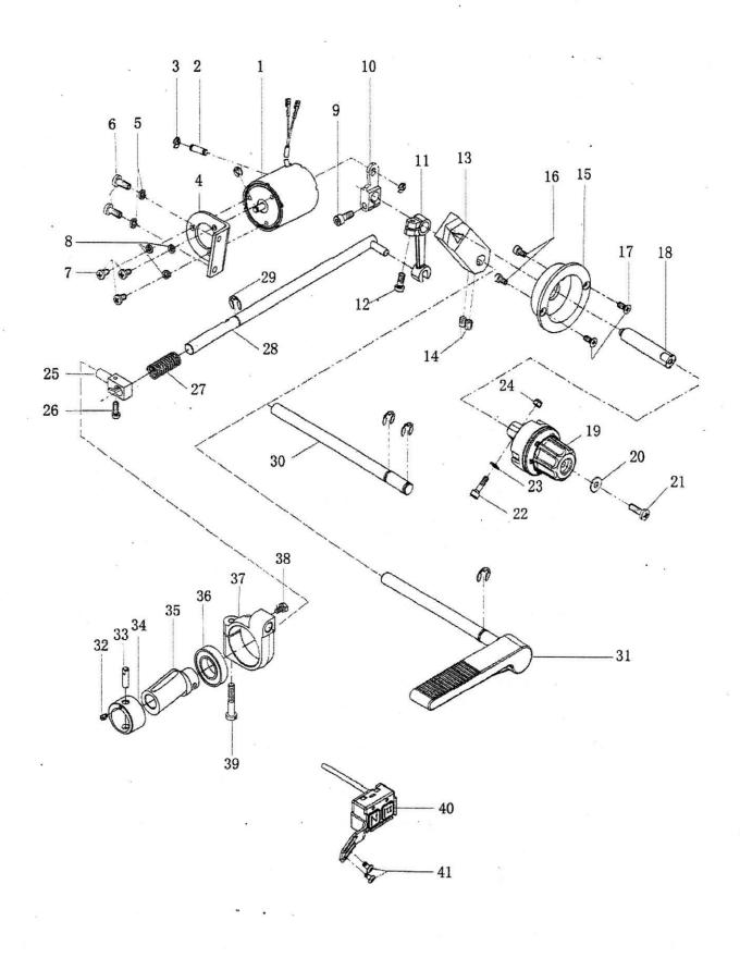
H.Lower shaft, feed dog and presseer foot lifting parts
